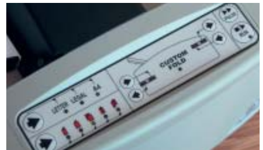
Automatic adjustment of the fold type by pushing a button on the display.
